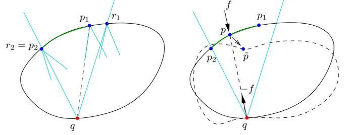
Fig. 2. Finding the segment of points forming a grasp with  $\mathbf{q}$ .
