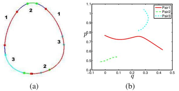
Fig. 5. Higher resolution yields one more pair of graspable segment on the second shape shown in Table I. The number of discretization points doubles from 500 to 1000.
