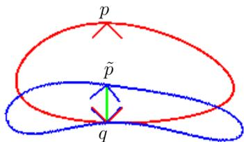
Fig. 6. The same finger placement  $\mathcal{G}(q, p)$  as in Fig. 4 retains the grasp under force of magnitude 0.6 and nonlinear elasticity modeling.
