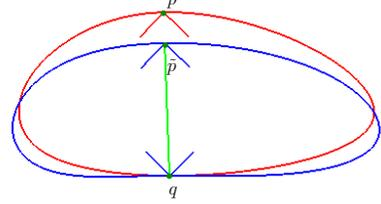
Fig. 4. Grasp  $\mathcal{G}(\mathbf{p}, \mathbf{q})$  of a closed cubic spline. Friction cones are drawn at the contact points.
