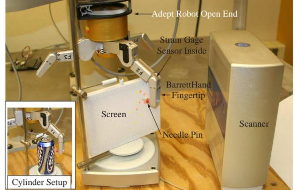
Fig. 4. Experimental setup with a screen and a cylinder.
